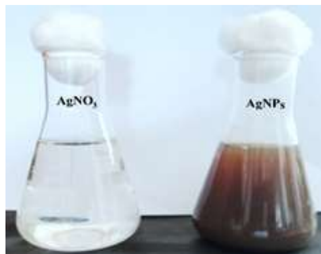
AgNO 3 = 1 mM AgNO 3 without Aristolochia bracteolata extract. AgNPs = 1 mM AgNO 3 with Aristolochia bracteolata leaf extract after 5 hrs of incubation (Brown colour)
