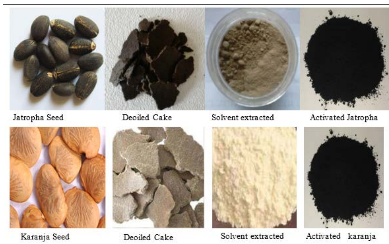
Fig 1: Deoiled Cakes of Jatropha and Karanja (Before and after activations)
