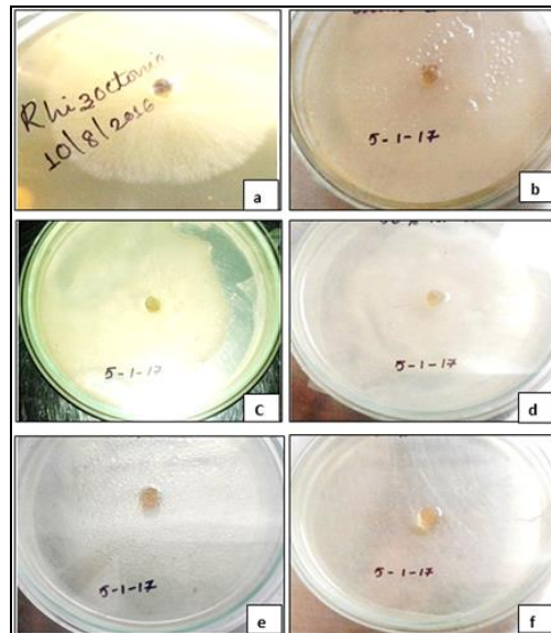
Fig 6: Evaluation of the antifungal activity against Rhizoctonia solani ; a. Control (Deionized water); b-e Rhizoctonia cultured in different concentration of CuONPs; b. 25 mg/L; c. 50 mg/L; d. 75 mg/L; e. 100 mg/L; f. 3mM CuSO 4
