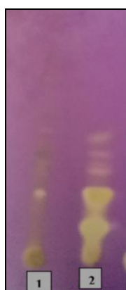
Fig 10: TLC plate of chloroform (1) and ethyl acetate (2) fractions obtained in toluene-ethyl formate-formic acid (5:4:1) in dally light after derivatization with 0.05% DPPH.
