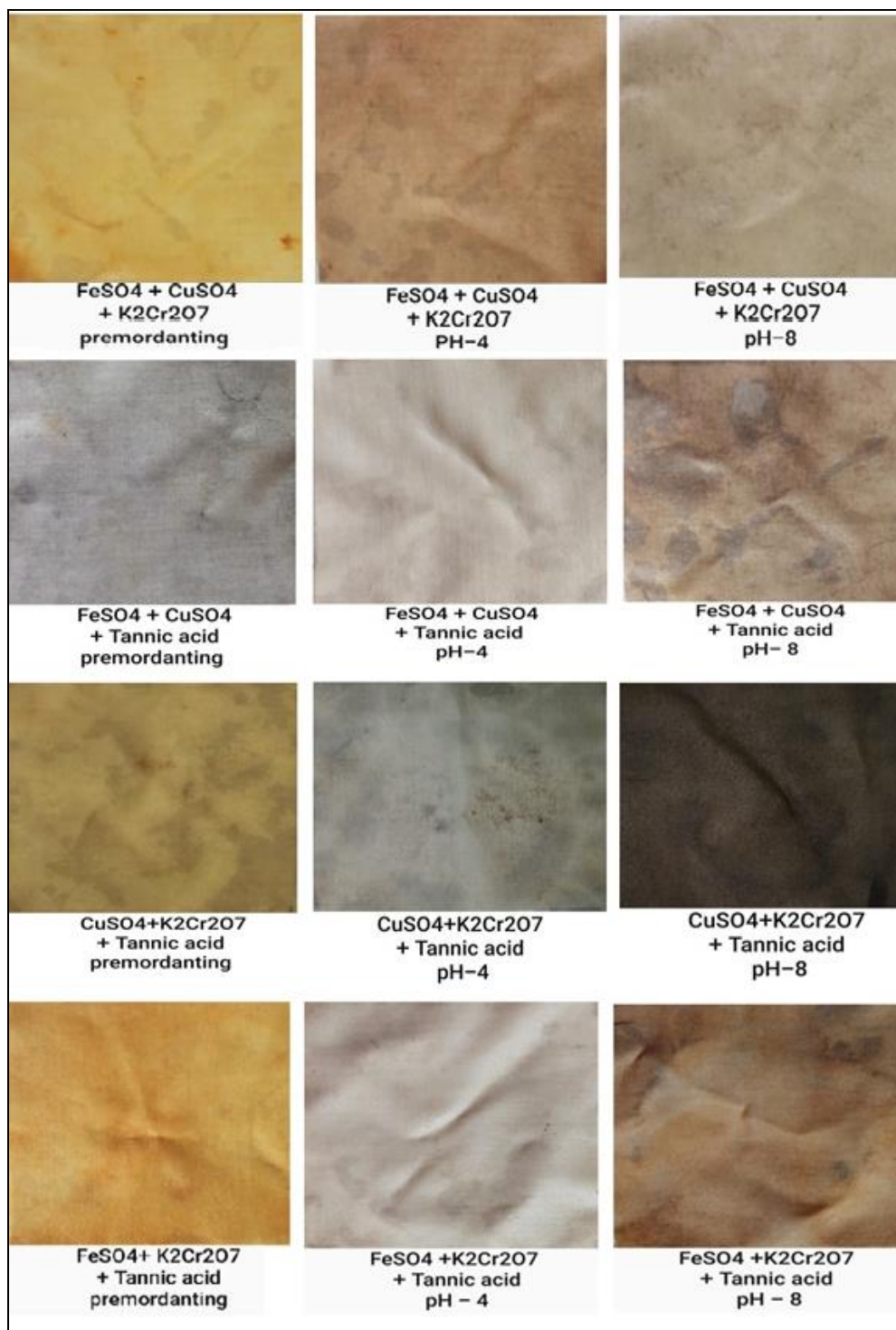
Fig 5: Colour shades produced by Premordanting of cotton with the combination of mordants and dyeing with crude dye solution of Mirabilis jalapa Linn. flowers.
