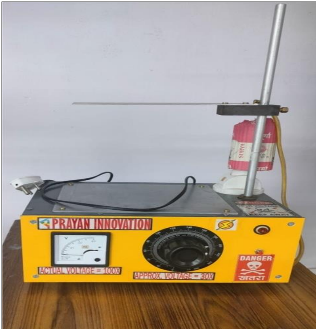
Fig 1: Equipment used for electric field treatment to algal cells
