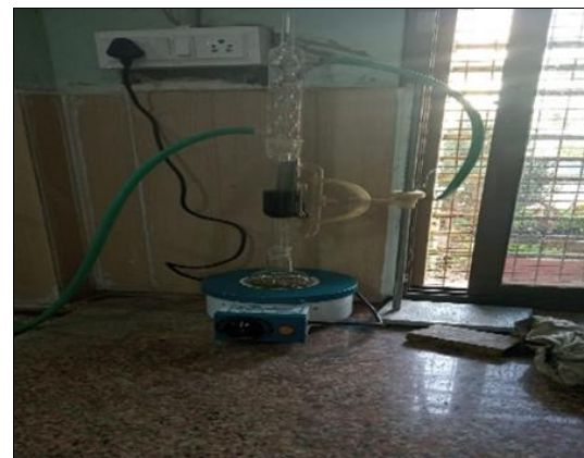
Fig 6: Extraction in Soxhlet apparatus
