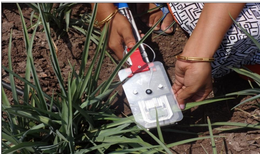
Fig 1: Measurement on gas exchange parameters using portable photosynthesis system
